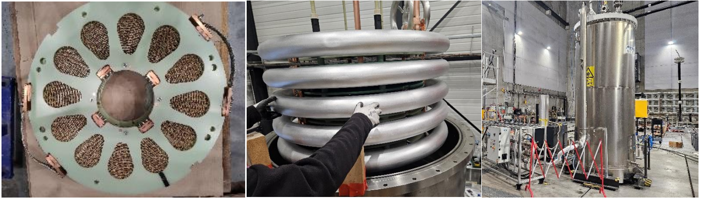
A pancake coil developed by SuperGrid Institute, containing 72 m of superconducting tape.
